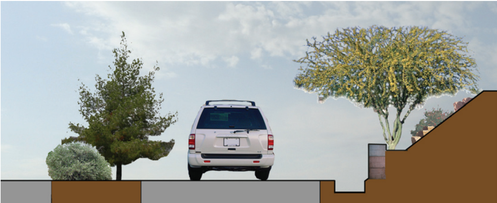
FRONTAGE ROAD FRONTAGE ROAD PLANTING STRIP ACCESS ROAD DRAINAGE SWALE BERM
