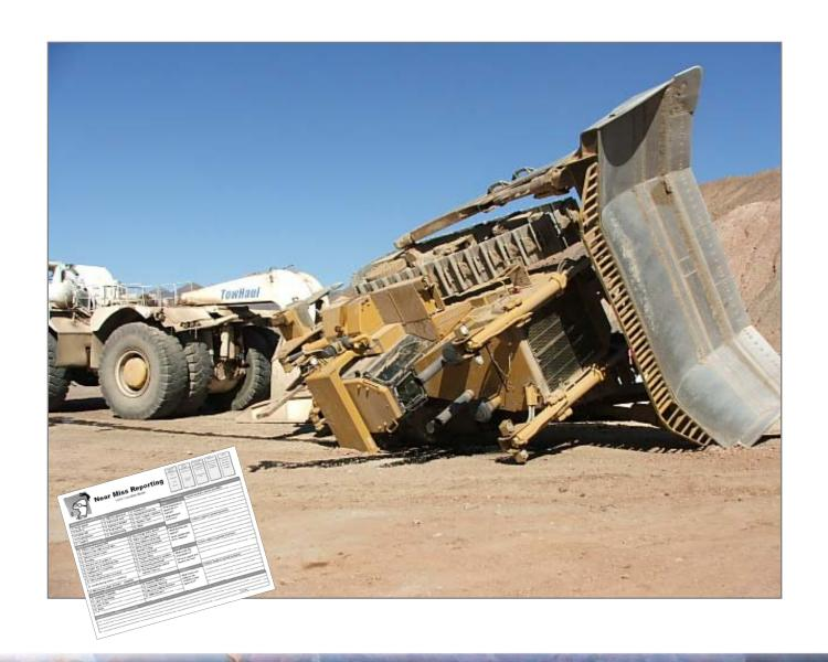
"Operator after loading dozer was going down a steep haul road. When he stopped at the bottom the dozer slid and fell off the trailer."
