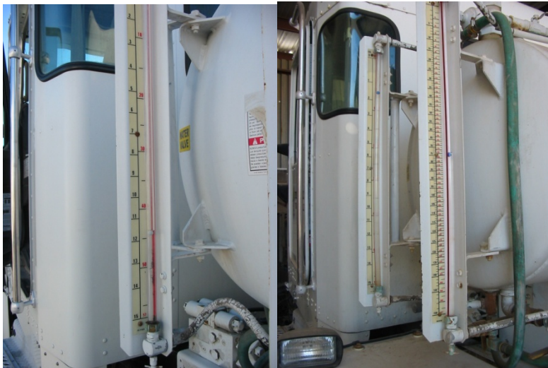
Figure 3: Legible Water Site Gauges
